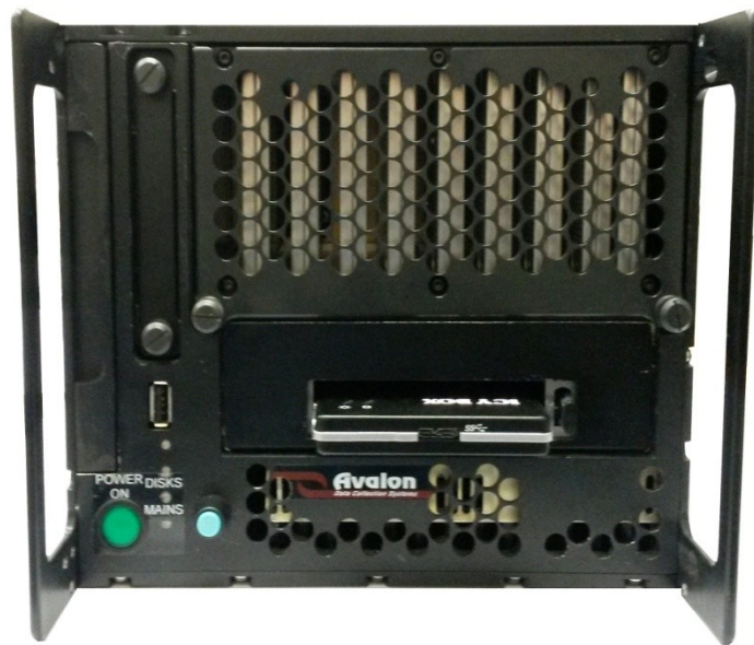
Avalon AE9000-8IF 8-channel 21.4 MHz IF SIGINT Disk Recorder with optional removable USB-3 disk drive (centre).
