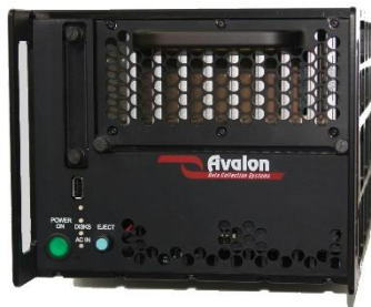
Avalon AE9000-100 Two-Channel SIGINT Disk Recorder (front view).
